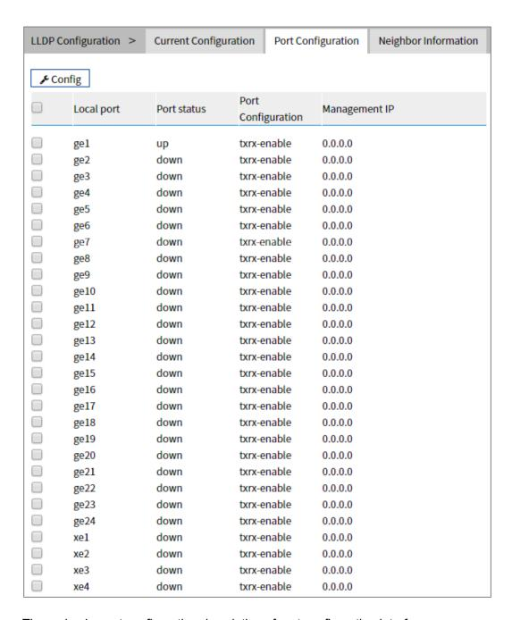
The main element configuration description of port configuration interface:
