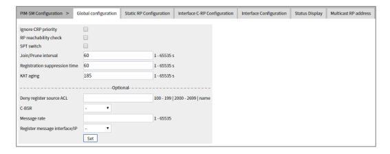
The main element configuration description of global configuration interface:
